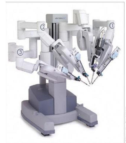
FIGURE 1. The da Vinci SI Surgical System
